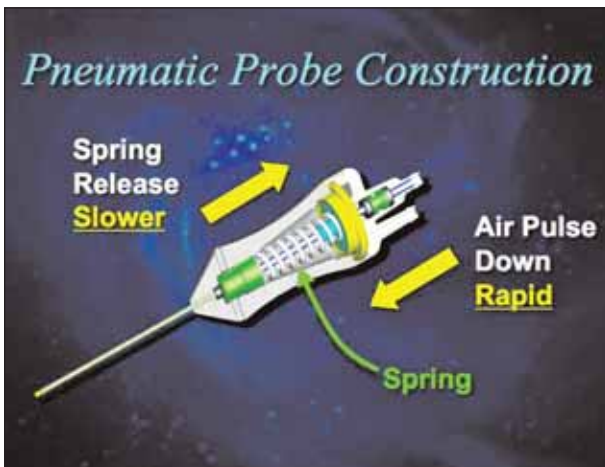
Figure 5. The spring-release mechanism slows cutting speed in the earlier pneumatic probe design.
