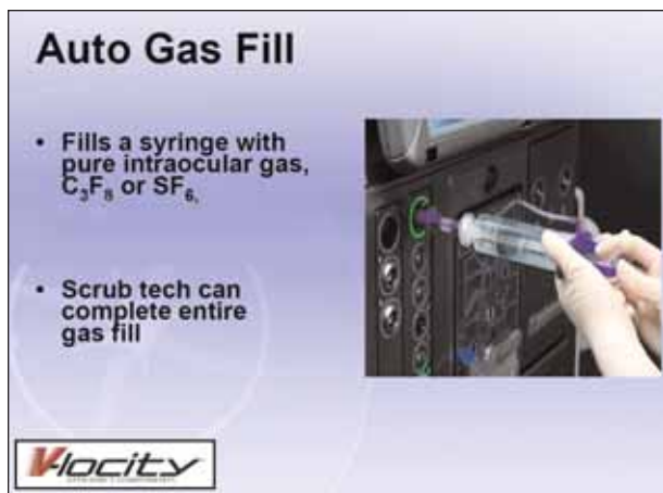
Figure 3. The auto gas fill mechanism is practical in terms of accuracy and cost savings.
